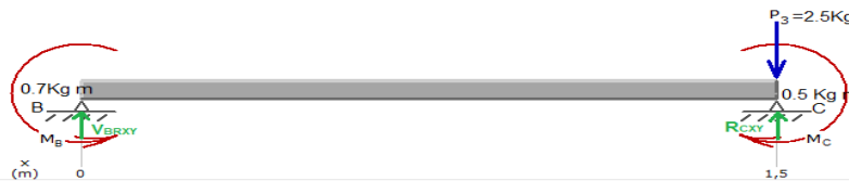
Fig. 2.11 Diagrama cuerpo libre tramo BC plano XY MDSolids.
